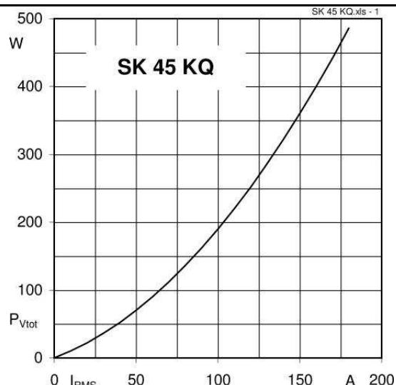
Fig. 1 Power dissipation per module vs. r.m.s. current
