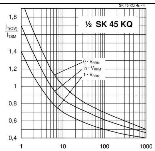
Fig. 4 Surge overload current vs. time
