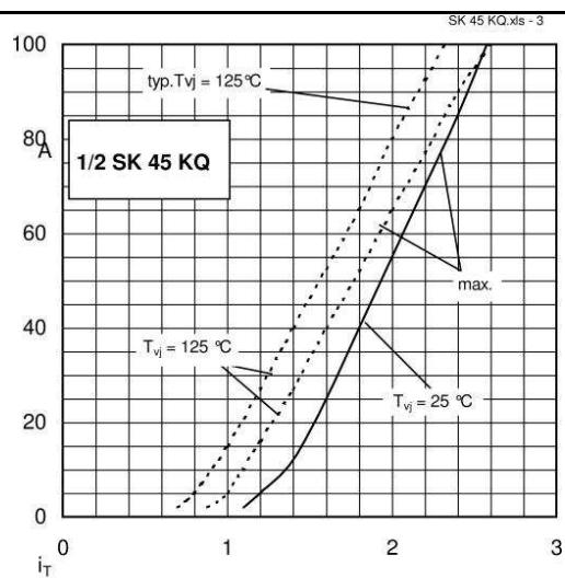
Fig. 3 On-state characteristics
