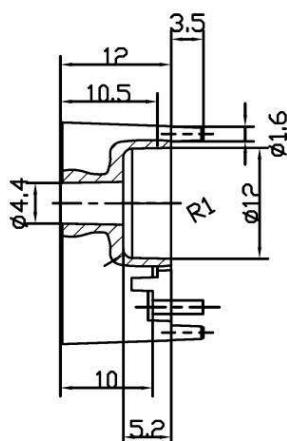
Case T 1 (Suggested hole diameter in the PCB for solder pins and mounting pins : 2mm)
